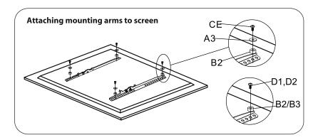
4. If your flat panel has a curved back or a recessed mounting point, spacers must be placed between the mounting arm and the flat panel to compensate the difference in depth.
